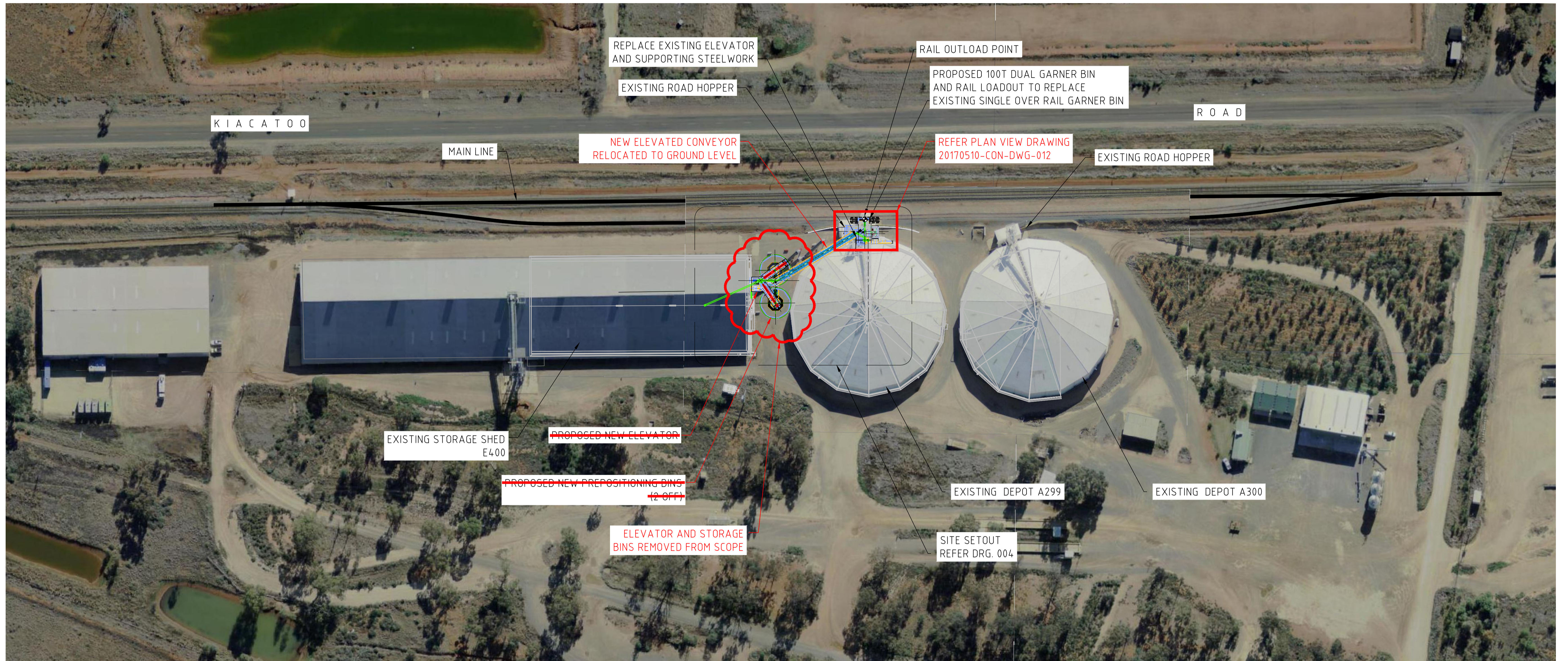
SITE LOCATION PLAN PROPOSED RAIL LOADING FACILITY SCALE 1:1000
